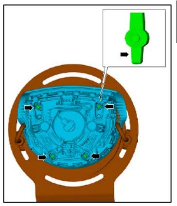
If a pin is damaged or has been lost, it can be replaced with a locking pin from the bag of spares included.
