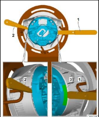
Remove locking pins <arrows> for horn ring with aid of longnose pliers.
