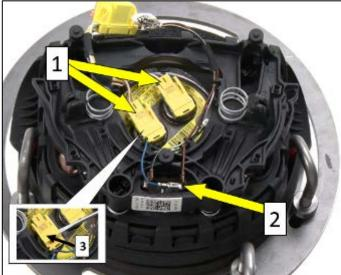
Clamp airbag centrally in airbag support. Securing points on the sides <arrows> and parallel, opposite each other.
