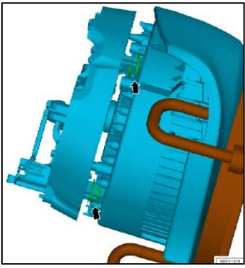
Position horn ring <arrows> with springs on securing clips and press firmly in place. Ensure that springs are seated correctly on both sides.
