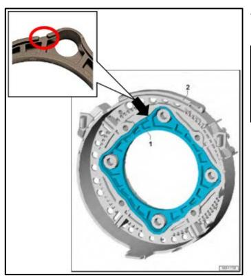
Fit insert ring <1> into horn ring <2>. The notch (circle) in the insert ring must be at top <arrow> when doing this.
