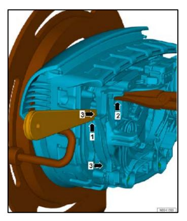
Apply removal wedge -3409- between horn ring and inflator <1> and press together locking elements using longnose pliers <2>.
