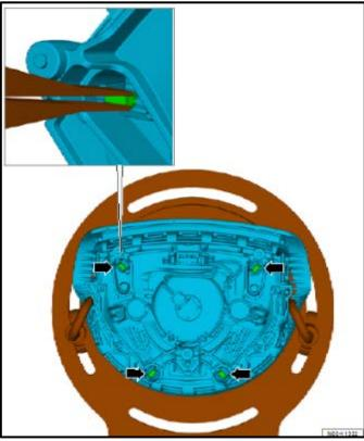
Remove locking pins <arrows> for horn ring with aid of longnose pliers.
