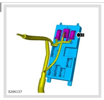
Disconnect the 3 electrical connectors from the BCM/GWM assembly.
