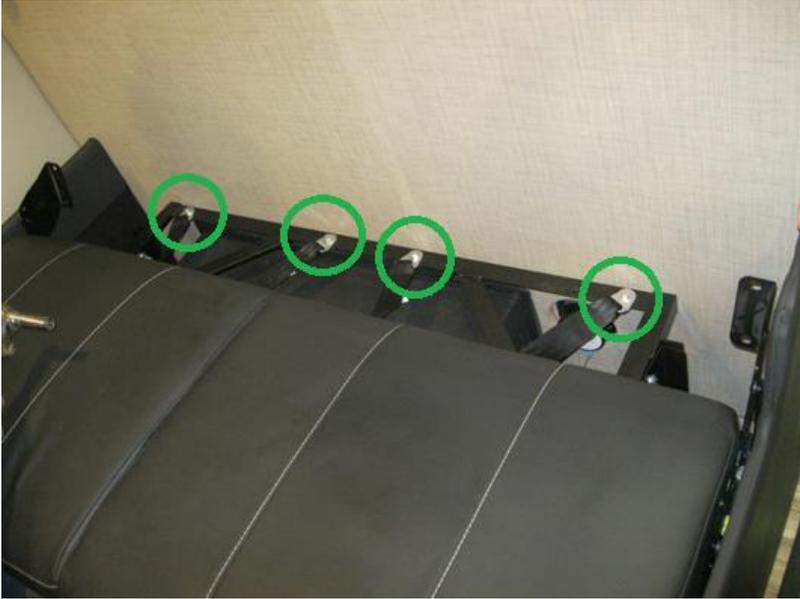
5. Add the Frame Reinforcement Angle (print TFM5493) on top of the seatbelt bracket with the bolt holes aligned. Position the vertical leg of the angle so it's against the sidewall. Reinstall the 2 seatbelts with 4 NEW 3/8"-16 x 1 1/2" grade 5 bolts as specified on the assembly drawing (print TFM5491). Use the included 3/8"-16 grade 5 nuts, flat washers, and lock-washers. Torque the 4 bolts to 18-25 ft-lbs.
