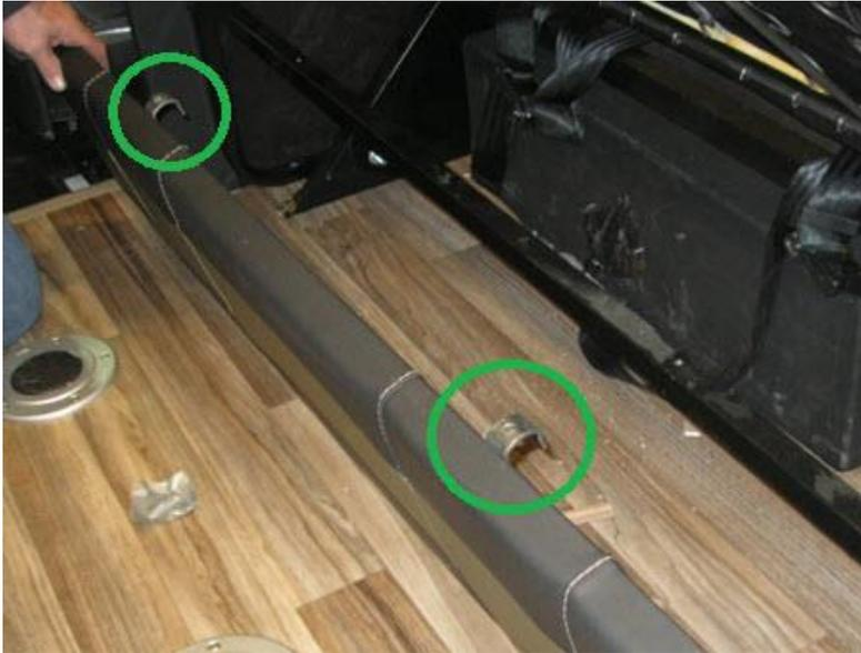
3. Remove the 4 nuts (2 per side) that secure the seat back to the sofa framing.
