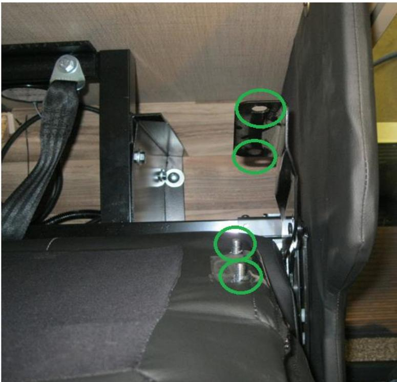
4. Remove and discard the 4 seatbelt bolts from the seatbelt bracket.
