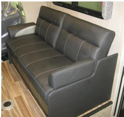
2. Remove the sofa arm rests, then lift the seat up enough to access and remove the screws securing the kickboard to the sofa frame.
