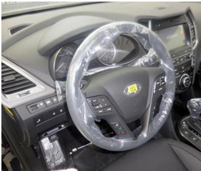
7. Reinstall the remaining components in reverse order of removal per the 2018 Santa Fe Sport or Santa Fe Service Manual (Steering System>Steering Wheel) and (Restraint >Airbag Module>Driver Airbag (DAB) Module and Clock Spring).
