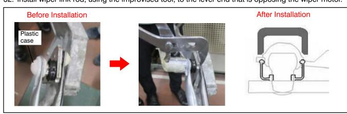
CAUTION The rubber seal must be properly seated. Confirm good condition of the rubber seal.
