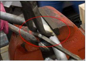
21. Use bent needle nose pliers to separate the wiper link rod from the wiper link assembly.
