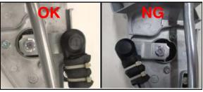
27. Install the wiper link plate to the wiper motor shaft. Make sure that the link plate and wiper link rod are in the correct orientation.
