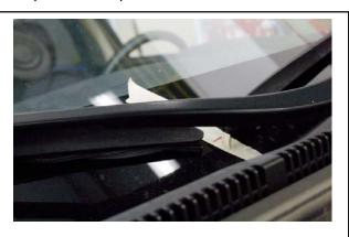
6. Remove the wiper arm blade assemblies.
