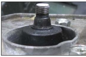
17. Check the knurling on the wiper motor shaft for any damage and/or debris. Clean off any debris with a clean rag.
