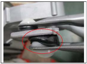
20. Pull back the rubber seal to prevent damage when performing the following steps.
