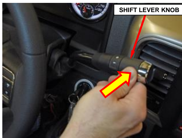
Figure 1 – Push Lightly On Shift Lever Knob Toward Instrument Panel To Feel BTSI Solenoid Pin Movement
