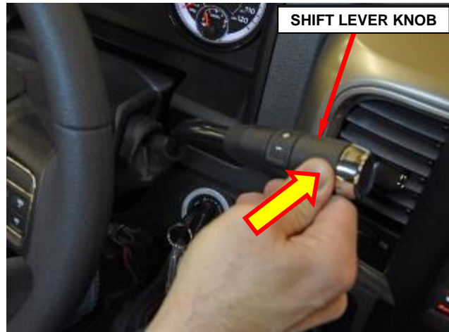
Figure 1 – Push Lightly On Shift Lever Knob Toward Instrument Panel To Feel BTSI Solenoid Pin Movement
