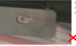
Airbag has been fitted under the rear roof trim and the retaining screw has perforated the airbag. The airbag must be replaced.
