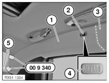
The airbag may be damaged by screw (2) located behind AIRBAG protective cap (4). To inspect the airbag for damage the rear roof trim (1) must first be removed, please follow repair instruction: 51 43 259 Removing and installing/replacing trim for rear roof pillar (D-pillar), left or right
