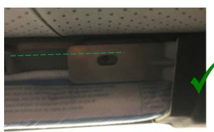
Airbag is installed correctly and the fixing screw has not perforated the airbag. No further action required.
