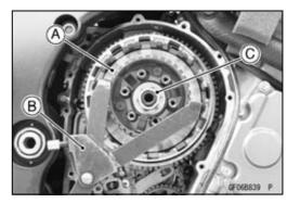
OUse the clutch holder with sharpened hook nose by grinding.
