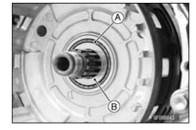
• Install the spacer [A] and the clutch hub [B]. OFace the stepped side [C] of the spacer to outside.
