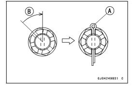
• Bend the cotter pin [A] along the nut [B].
