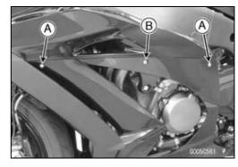
Pull the rear part of the lower fairing downward to clear the hooks [A] from the upper fairing [B].
