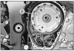
Remove: Needle Bearing [A] Sleeve [B]
