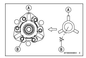
Install the fourth torque limiter spring [A].
