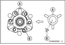
Install the second torque limiter spring [A].
