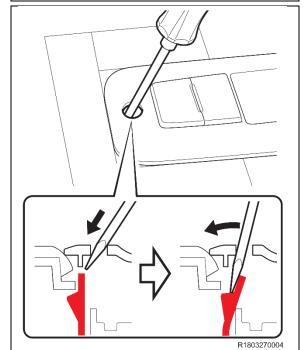
e) Using a small screwdriver, release the locking tab by inserting the screwdriver into the hole and prying the tab back.
