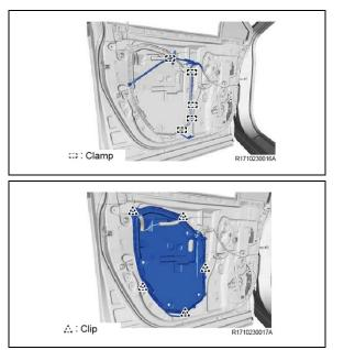
c) Disengage the 5 clamps.
