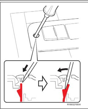
e) Using a small screwdriver, release the locking tab by inserting the screwdriver into the hole and prying the tab back.
