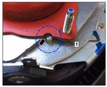
• Install the new inflator onto the studs.
