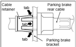
2. Fit a hose clamp over the parking brake cable retainer.
