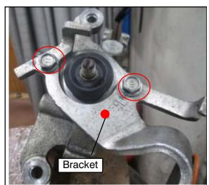
9. Unbolt and remove the bracket.
