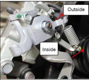
a. Engage the hook of the spring from "inside" to the "outside" direction.
