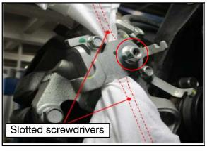
6. Insert (2) slotted screwdrivers diagonally, and remove the lever by lifting it with the tips of the screwdrivers.
