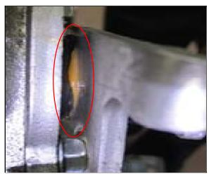
NOTE: There is no need to wipe off excess grease that flows out of the boot after the lever has been tightened (Grease overflows as the boot is filled with a sufficient amount, and therefore, this is not an issue.)
