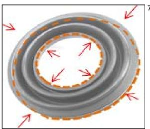
7. Apply the grease to the inner and outer races of the piston boot, as shown on the dotted lines.
