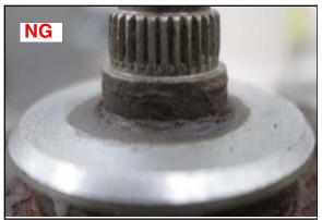
b. If rust has reached the caliper body surface and/or rust is observed on the flange surface inside the boot, obtain a new Caliper Body Assembly and proceed to INSTALL CALIPER BODY ASSEMBLY (page 25).
