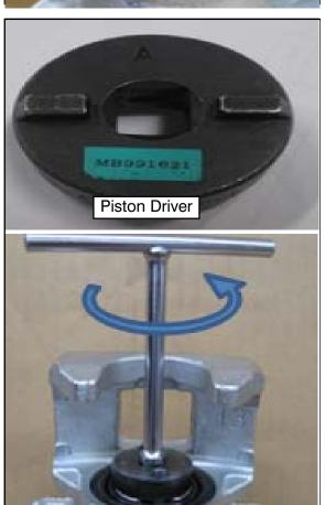
3. Use a Piston Driver and rotate counterclockwise to remove piston assembly from the caliper.
