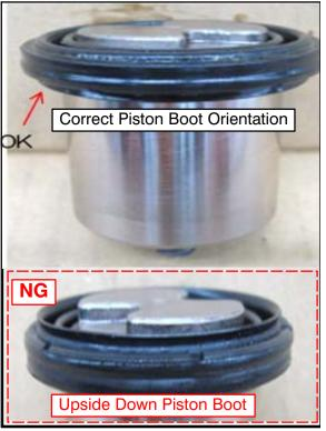
8. Install the new piston boot to the piston assembly.
