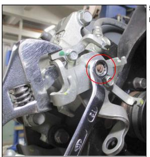
5. Loosen, but do not remove, the nut.
