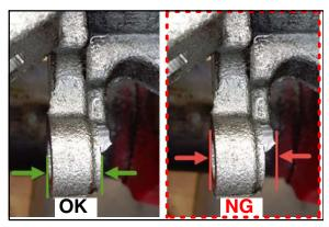
Clamp the caliper body assembly with a vise, at the illustrated section. (Only if caliper body has been removed, on page 7.)
