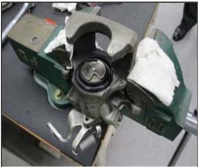
1. Clamp the caliper body assembly in the vise.
