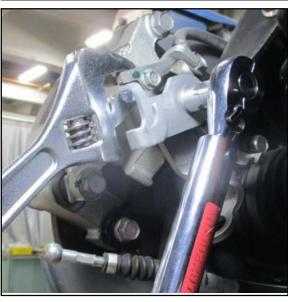
13. Tighten the **original nut** (after grease application) to **21 ft—lb (29 Nm)**.
