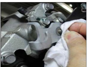
17. Remove and discard the **original nut**, and wipe off the grease on the thread of the operating shaft with dry, clean rags.
