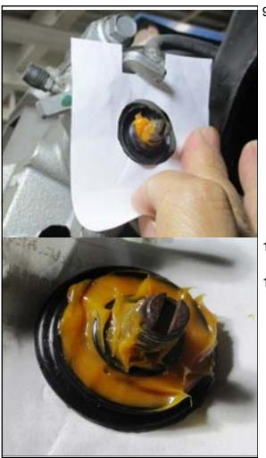
Use a masking sheet to prevent grease from spreading to the surrounding surfaces and apply grease on the outside of the lever boot (0.5 g).
