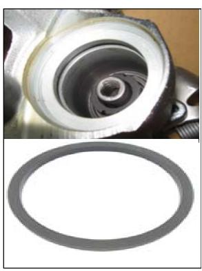
5. Remove the piston seal.
