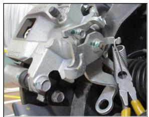
1. Unhook the spring from the lever, using needle nose pliers.
