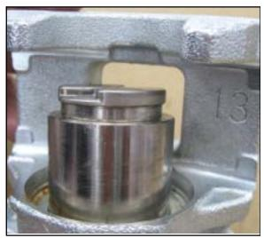
4. Pull up and remove the piston.
