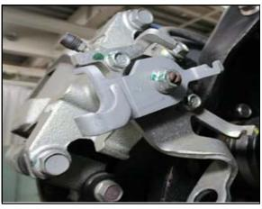
15. Confirm that the caliper lever is at the original position after it is assembled. (The clearance between the lever and stopper must be 1 mm or less.)
