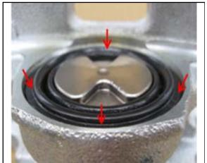
10. Fit the piston boot outer race to the caliper body gap.
