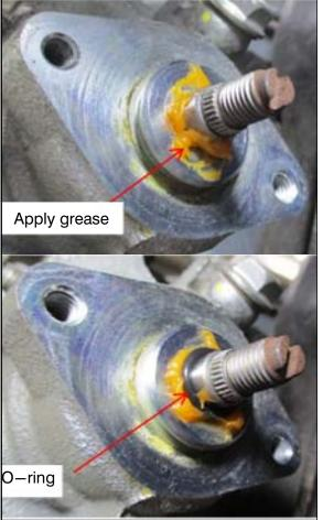
4. Apply grease, included in the lever and boot kit, onto the caliper body around where the operating shaft is inserted, and set the O-ring, included in the lever and boot kit, onto the operating shaft.
