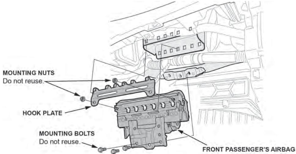
3.5. Remove the front passenger's airbag.
