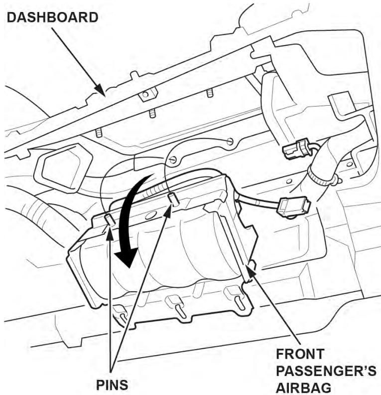
17.2. Install the front passenger's airbag using the new mounting bolts and the new mounting nuts.
