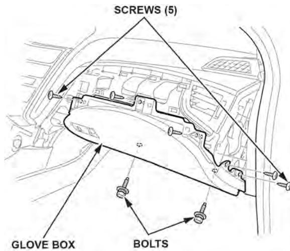
3.2.3. Remove the glove box by pulling it by hand to detach the clip.
