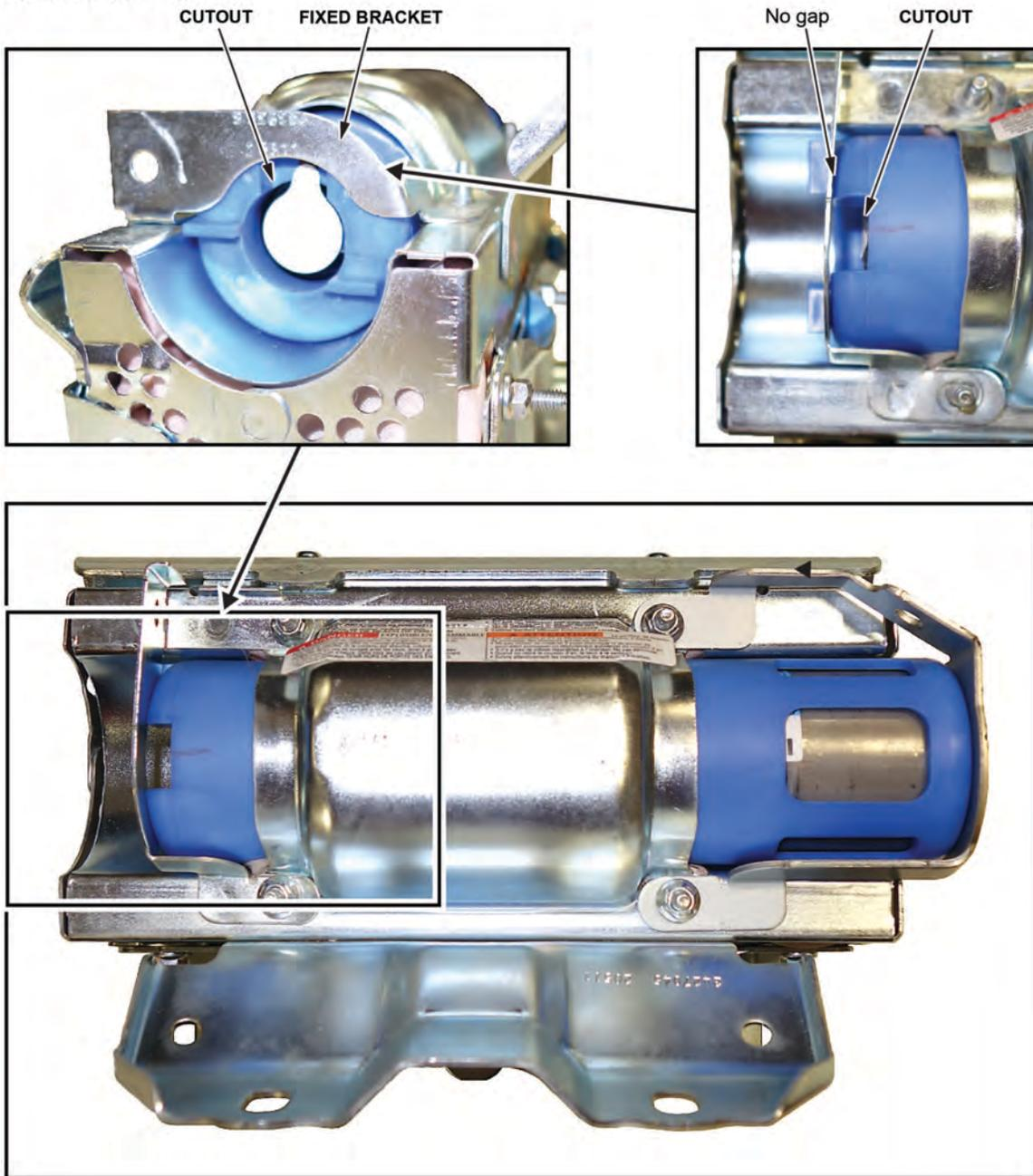
12.3. Install the bracket included in the kit onto the airbag module. Check there is no space or gap between the inflator and bracket by pushing the bracket against the inflator.
