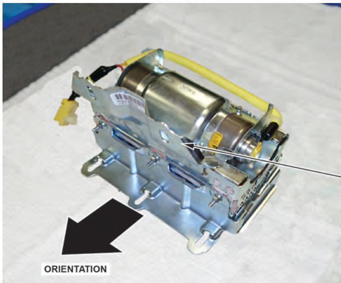
5. Visually inspect the airbag and the inflator for any unusual writing or markings. Refer to IDENTIFYING COUNTERFEIT AIRBAGS.
