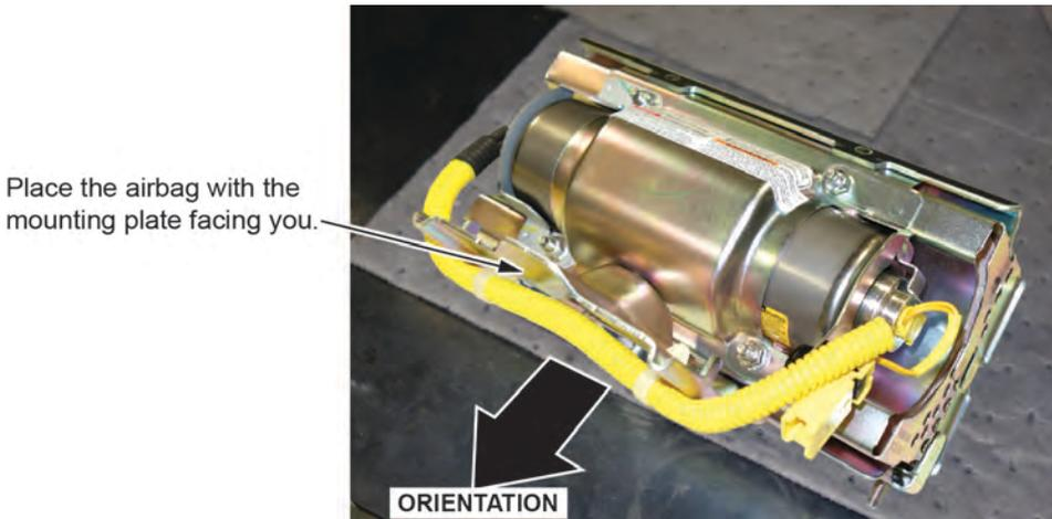
5. Visually inspect the airbag and the inflator for any unusual writing or markings. Refer to IDENTIFYING COUNTERFEIT AIRBAGS.
