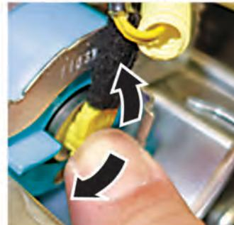
15.3. Connect the yellow wire connector to the connector on the side with the long plastic collar.
