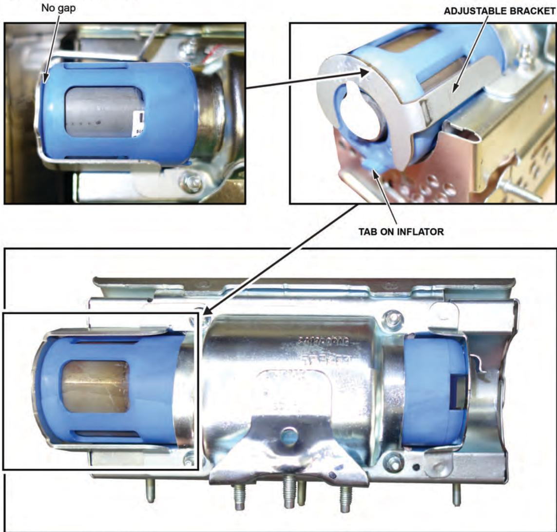
13. Hold the bracket against the inflator, then install the new 5 mm locknuts and torque them in sequence to **3.9 N·m (34 lb-in)**.
