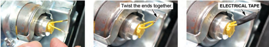
8.3. Tape the twisted ends with electrical tape.
