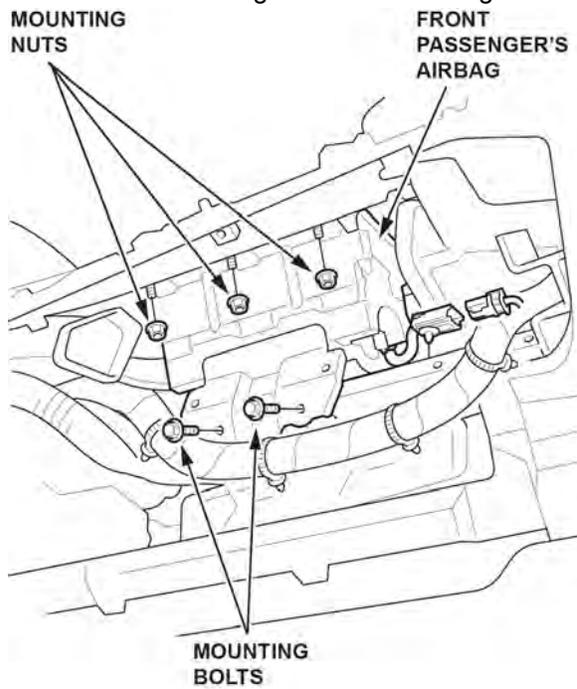
3.6. Release the pin and remove the front passenger's airbag.
