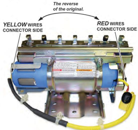
15.2. Connect the red wire connector to the connector on the side with the short plastic collar. Align the "T" shape in the inflator harness connector with the T-shaped inflator connector, then press the connector into place.
