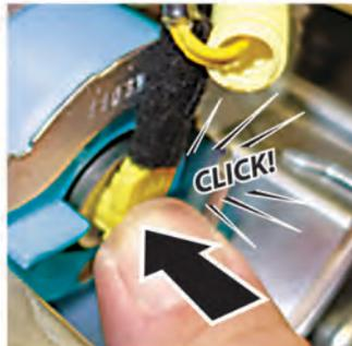
③ Wiggle the connector to make sure it's secure.
