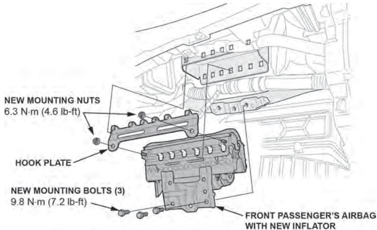
17.2. Torque the mounting nuts and bolts to the following specifications:
