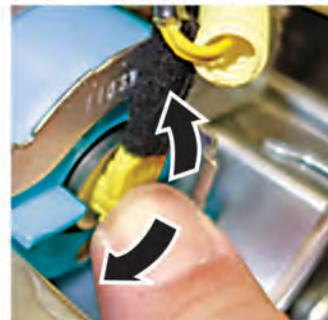
15.3. Connect the yellow wire connector to the connector on the side with the long plastic collar.
