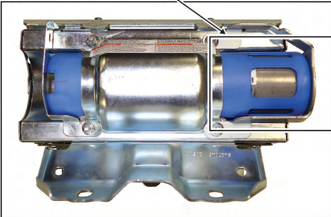
13. Hold the bracket against the inflator, then install the new 5 mm locknuts and torque them in sequence to **3.9 N•m (34 lb-in)**.
