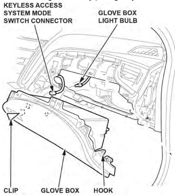
3.2.4. While holding the glove box, disconnect the glove box light connector and the keyless access system mode switch connector (if equipped).
