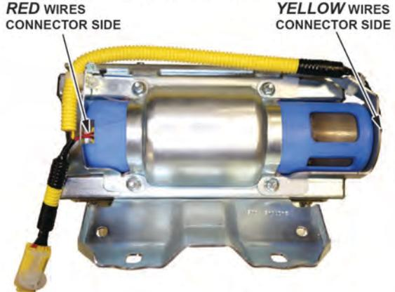
15.2. Connect the red wire connector to the connector on the side with the short plastic collar. Align the “T” shape in the inflator harness connector with the T-shaped inflator connector, then press the connector into place.
