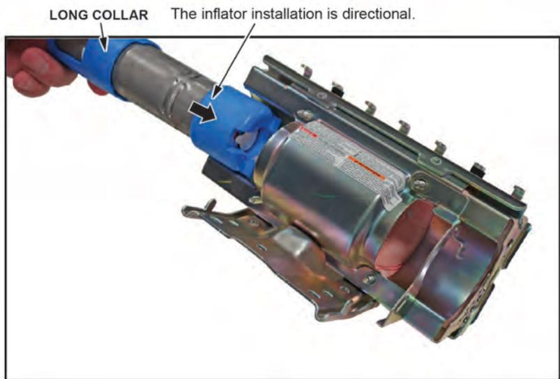
12.2. Slide the inflator in until the plastic collar contacts the bracket. The two tabs should align with the side of the airbag module and the metal tab as shown. There should be no space or gap between the inflator and bracket.
