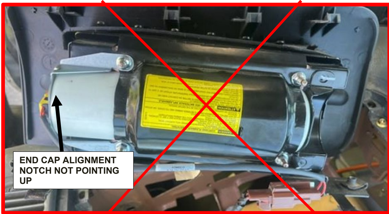
FIGURE 3 – NO GOOD (NG) INCORRECT ORIENTATION OF END CAP
