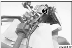
Mount new sealing cup 🕑 on the push rod of the hand brake lever.
