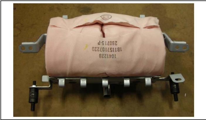
b) Mount the adaptors (579943-3R3) to the airbag as shown.
