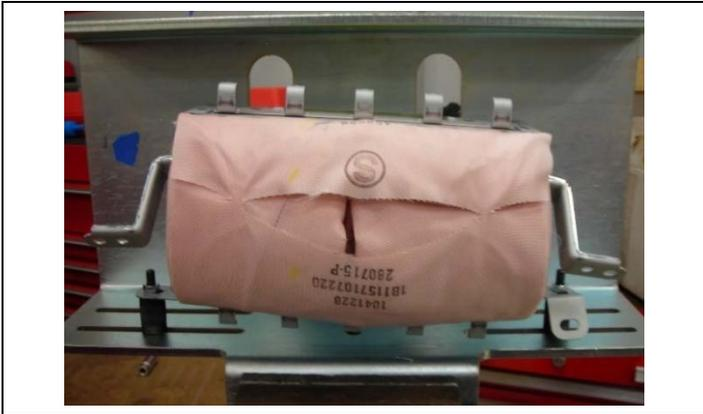
c) Mount the airbag to the mounting bracket as shown.
