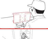
ALWAYS keep as much of your body as possible in front of the bracket when working on the airbag assembly.
