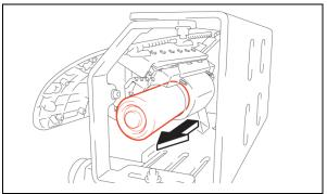
b) Remove the inflator from the airbag assembly and place it on a safe work surface.
