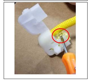
c) Open the connector cover. Once open carefully use a pocket screwdriver to disengage the release tab and remove the connector cover from the connector
