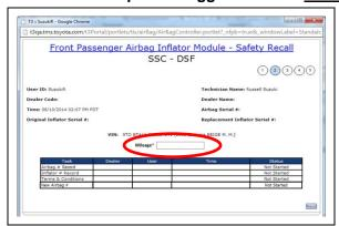
e) Record the vehicle mileage into the serial number recording application.
