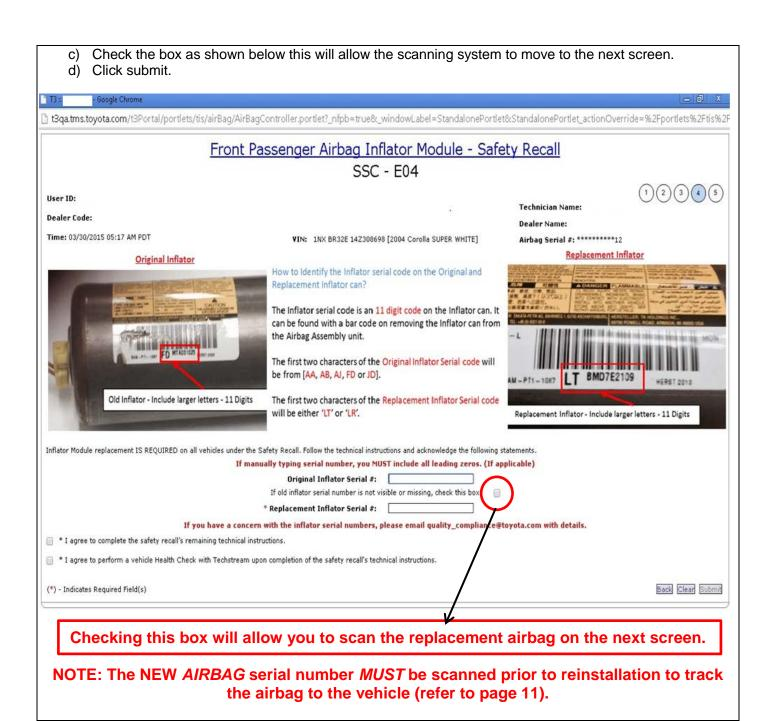
e) Scan the NEW airbag barcode in the Serial Number Recording Application.
