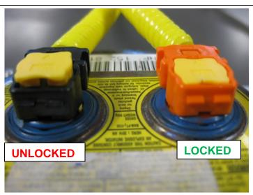
NOTE: Ensure the secondary locks are fully engaged.
