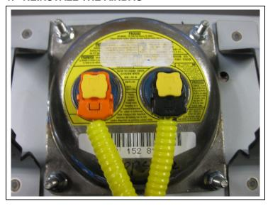
a) Install the new harness onto the new airbag by plugging in the two connectors.
