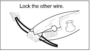
c) Set the other wire in the electro tap and lock it in place using pliers.
