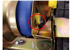
c) Confirm the harness is not pinched by the stopper plate
