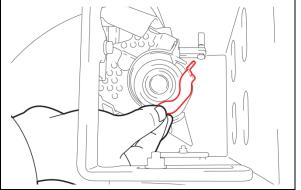
b) Remove the stopper plate and place in a secure location because it will be reused.
