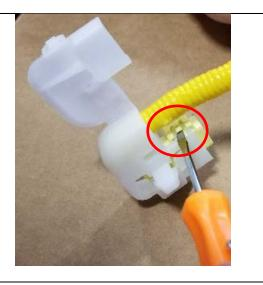
c) Open the connector cover. Once open carefully use a pocket screwdriver to disengage the release tab and remove the connector cover from the connector
