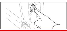
If the anti-static kit is not available, before starting work and periodically while working on the vehicle, touch a metallic part of the vehicle to discharge static electricity in the body.
