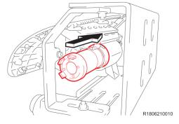
b) Carefully slide the new inflator into the airbag assembly.
