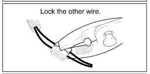
c) Set the other wire in the electro tap and lock it in place using pliers.
