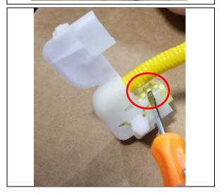
c) Open the connector cover. Once open carefully use a pocket screwdriver to disengage the release tab and remove the connector cover from the connector
