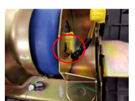
c) Confirm the harness is not pinched by the stopper plate
