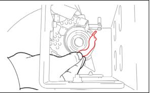
b) Remove the stopper plate and place in a secure location because it will be reused.
