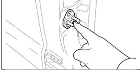
If the anti-static kit is not available, before starting work and periodically while working on the vehicle, touch a metallic part of the vehicle to discharge static electricity in the body.
