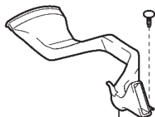
NO. 2 CONSOLE BOX DUCT
