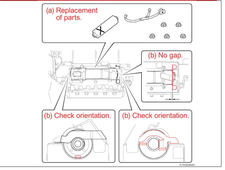
k) Tighten the 5 nuts evenly in several increments in the sequence shown. Use a socket driver or torque wrench to tighten the nuts.
