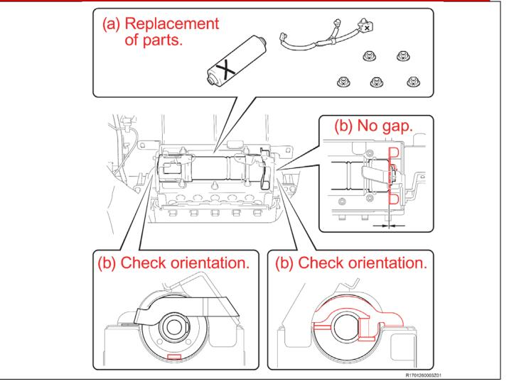
k) Tighten the 5 nuts evenly in several increments in the sequence shown. Use a socket driver or torque wrench to tighten the nuts.
