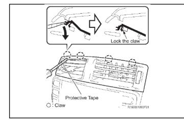
Removing the No. 3 air register
