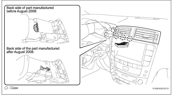
Using your finger on the right side push out at the point shown to disengage the 3 claws and remove the register from the instrument panel.
