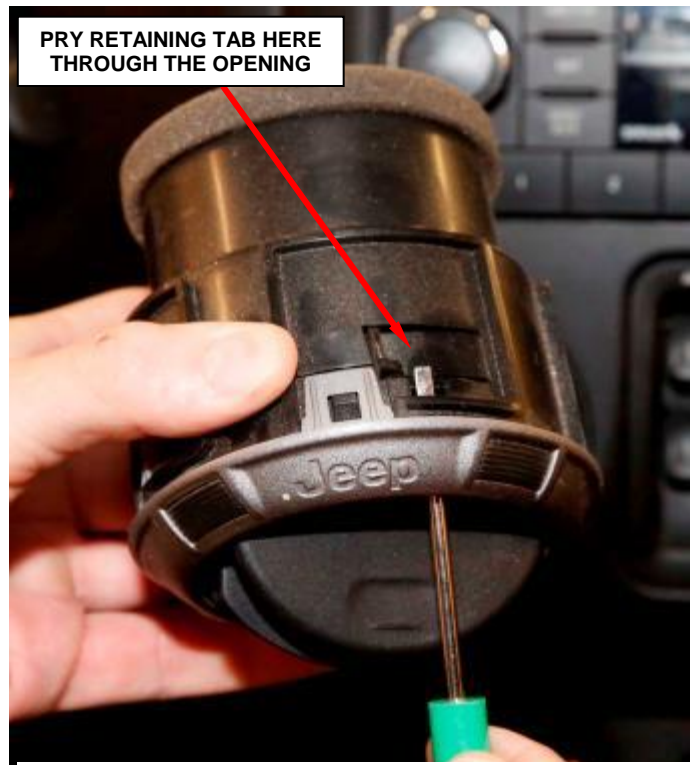
Figure 121 - HVAC Outlet Tab
