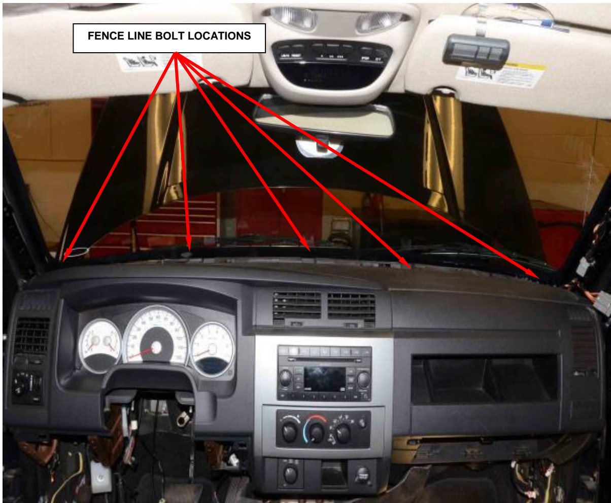
Figure 100 - Fence Line Bolts
