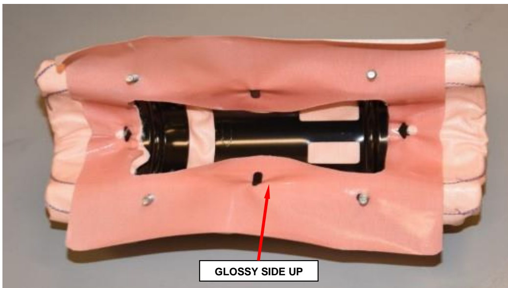
Figure 132 – Fabric Gasket to Cushion (Glossy Side Up)
