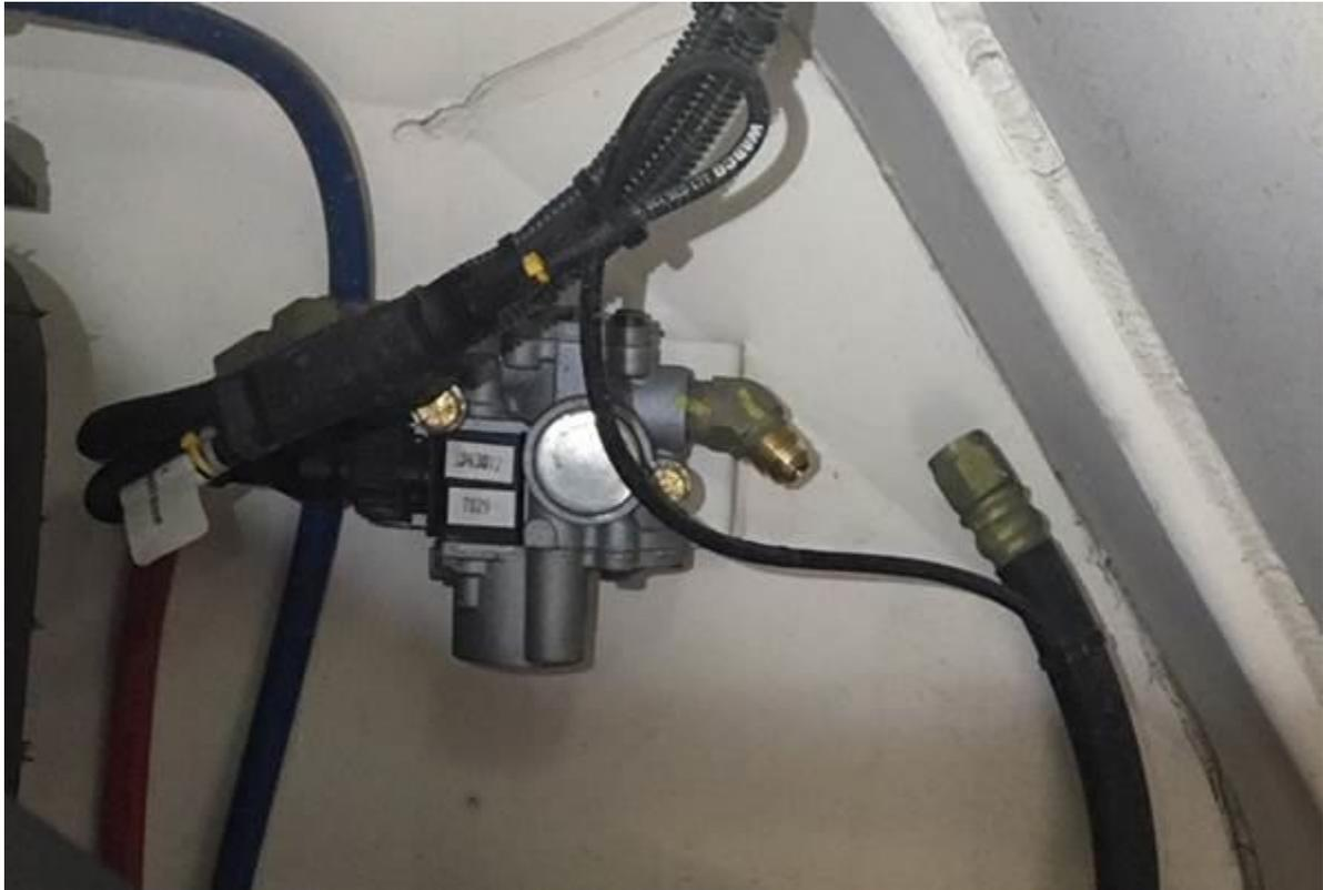
**Figure 2: Disconnect brake hose from 45-degree fitting**
