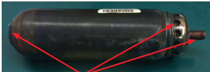
The shape, holes, and copper-colored stud indicate this not a Genuine Subaru inflator.
