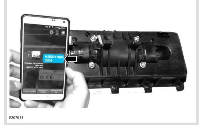
Use a smartphone with a QR scanner application to scan the QR code on the passenger airbag module label.
