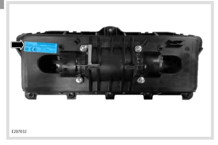
Locate the label on the rear side of the replacement passenger airbag module.
