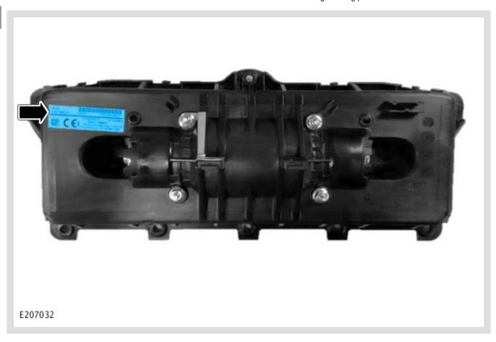
Locate the label on the rear side of the replacement passenger airbag module.
