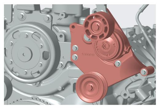
Install new tensioner bracket 5572555. See below figure for capscrew part numbers and torque specification.
