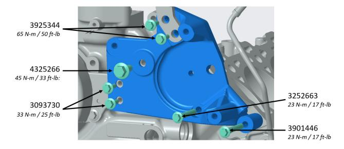
Install belt tensioner 4316721 using capscrew 4324936. Torque: 65 N-m [ 50 ft-lb]
