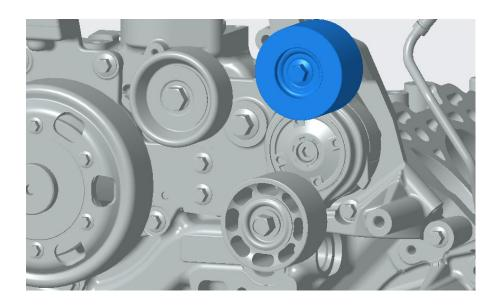
Install idler pulley assembly 5598324 (integrated capscrew). Torque: 65 N-m [ 50 ft-lb]
