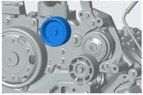
Install idler pulley assembly 5598353 (integrated capscrew). Torque: 65 N-m [ 50 ft-lb]
