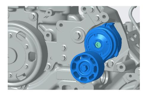
Install idler pulley assembly 4390737 (integrated capscrew). Torque: 34 N-m [ 25 ft-lb]
