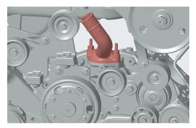
Install thermostat into new thermostat housing 5414320. Install thermostat housing 5414320 as shown in the figure below. Use same capscrews 4325276. Refer to procedure 008-157-tr. Torque: 18 N-m [ 159 in-lb]
