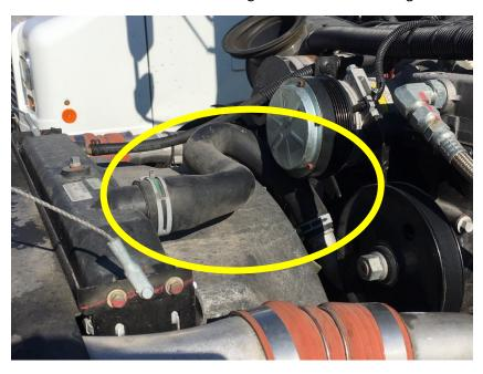
Remove thermostat housing 4335418. Retain capscrews (4325276). Retain thermostat.
