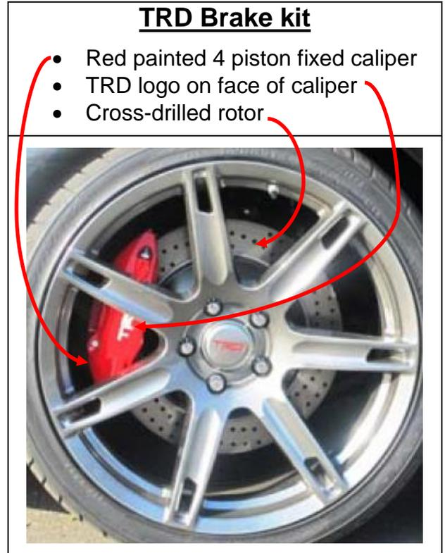
Note: TRD wheels may be found on vehicles without the TRD Brake kit. This Safety Recall only involves the TRD Brake kit.
