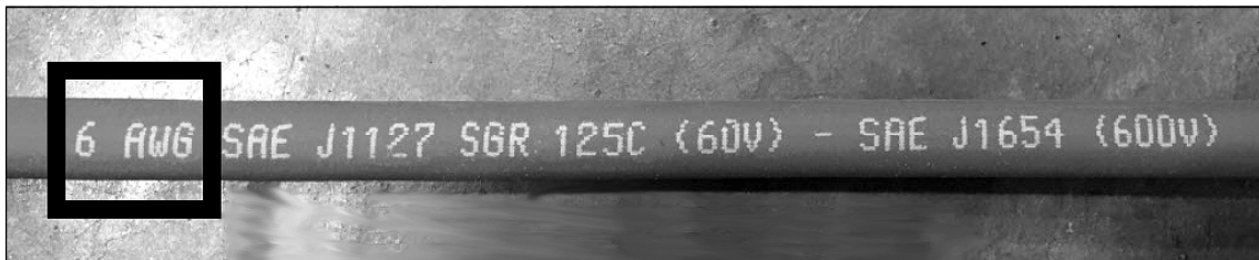
Figure 3 — 6 AWG Wire Identification
