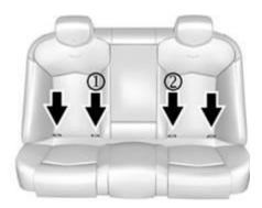
The presence of hardened adhesive on the lower child-seat anchor bar(s) may cause portions of the bar(s) to be too large in diameter, interfering with child seat installation efforts.
