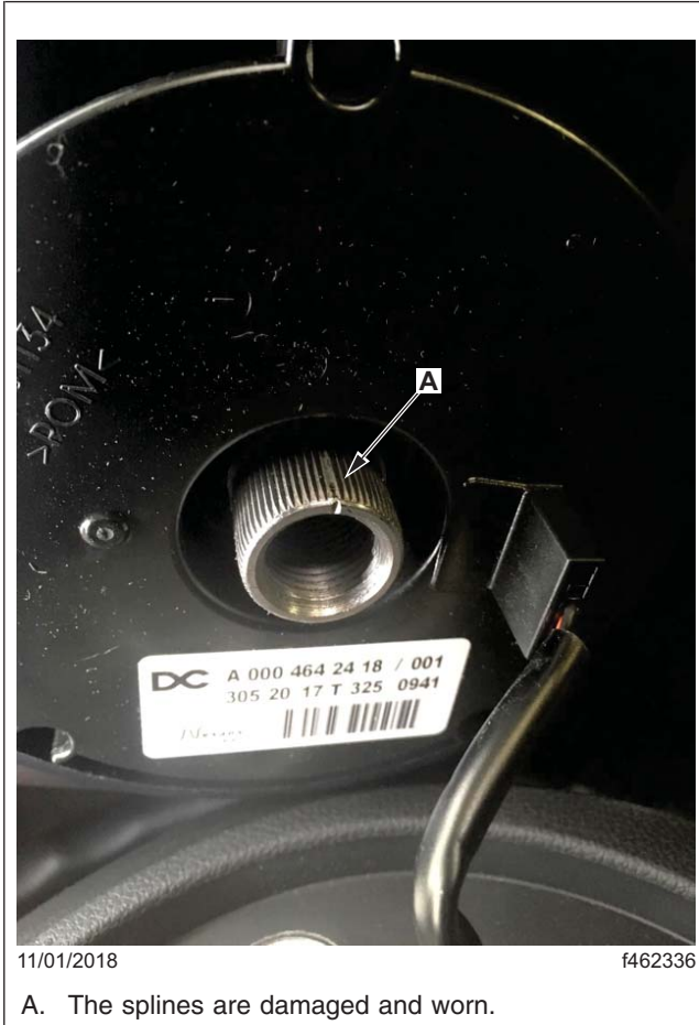
Fig. 4, Damaged Steering Column Splines
