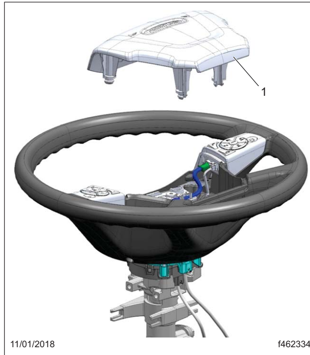
Fig. 3, Removing the Steering Wheel Cover
