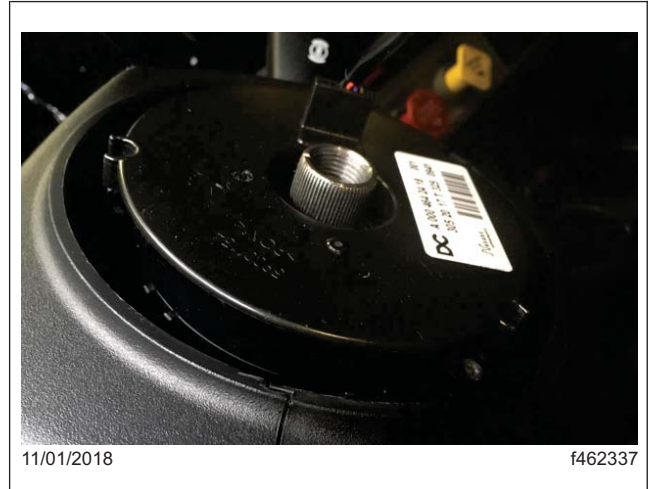
Fig. 5, Steering Column Splines with Undamaged Grooves
