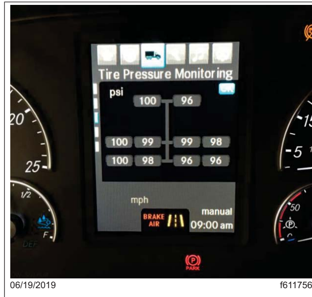
Fig. 23, ICUC Tire Pressure Monitoring Screen
