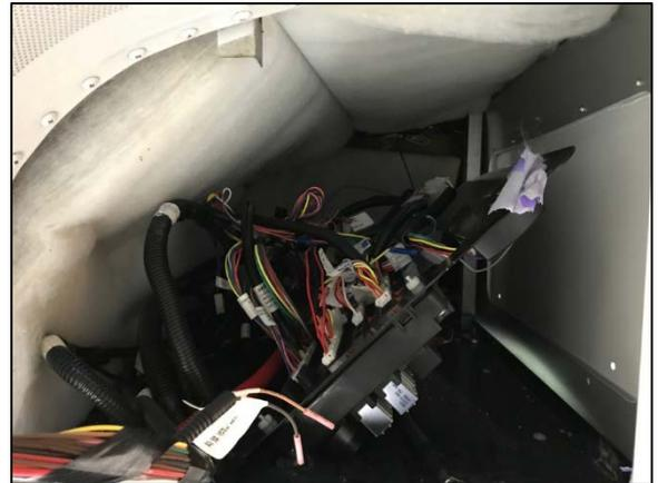
**Figure 6: Back of PC Boards After Side Cushion is Removed**
