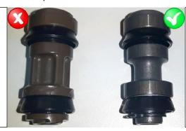
The new machined aluminum front brake master cylinder piston is shown on the right.
