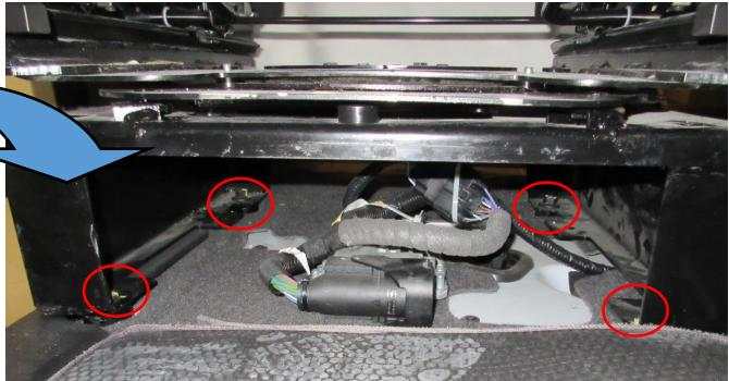
Apply 59ft.-lbs (80Nm) torque to all four pedestal to floor bolts.
