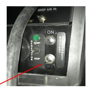
3. Turn off chassis battery disconnect at driver side shore cord access door.
