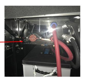
Note: If your coach is equipped with electric engine bay latches, ensure that the passenger side engine access door is open prior to turning off chassis batteries.
