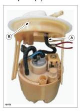
4. Remove the fuel pump, fuel filter, pressure regulator and transfer jet pump as a single unit from the reserve cup (A) while pressing the snap fit tab (B) using a flathead screwdriver.
