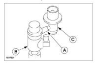
**NOTE:** Insert the tip of the flathead screwdriver into the position indicated (A) and rotate the screwdriver to pry up the pressure regulator (B) with the transfer jet pump (C).
