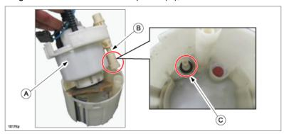
f. Determine whether to reuse the reserve cup if damaged, depending on the condition of the damage.
