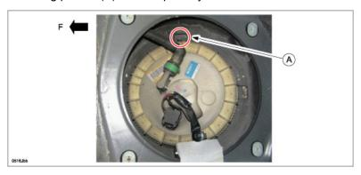
c. While keeping the alignment mark and the retainer notch aligned, tighten the fuel pump ring to the rotation angle (50-140 degrees) and specified torque (80-135 Nm, 8.2-13.7 kgfm, 59-99 ft lbf) using the SST. Total angle for step 2 and step 3 is 410-500 degrees: One full rotation (A) and tighten so the start position (3 ribs) comes to the star mark (B) using the SST (F=front of vehicle).
