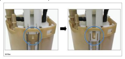
b. Engage the snap fit tab (A) and set plate arm (B), and verify that it is properly engaged to the reserve cup (C).
