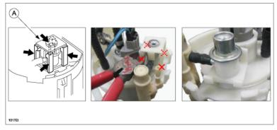
6. Remove the pressure regulator and transfer jet pump from the fuel filter (high-pressure) by using the flathead screwdriver.
