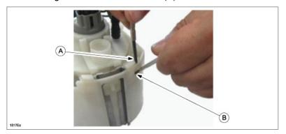
e. Remove the fuel filter (high-pressure) (A), pressure regulator and transfer jet pump (B) as a single unit from the reserve cup.
