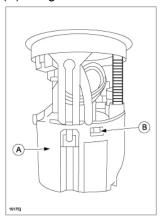
**CAUTION:** When disengaging the snap fit tab, DO NOT hold the reserve cap as shown. This is to avoid injury if small flathead screw driver slips and comes down unintentionally.
