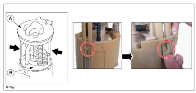
2. Disconnect the fuel pump connectors (A).
