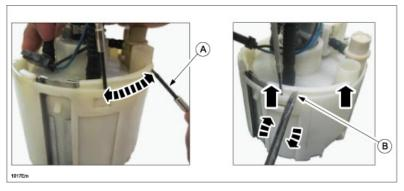
c. Insert the flathead screwdriver in the snap fit tab (A) and pry up, lifting the fuel filter (high-pressure) (B).
