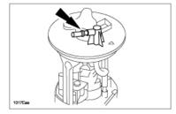
**CAUTION:** Be careful not to break the set plate arm by applying excessive pressure. If it is broken, it could cause a fuel pump unit operation malfunction (A=set plate, B=fuel filter (high pressure)).
