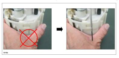
a. Insert the 2.0 mm flathead screwdriver at the snap fit tab (A) and disengage the snap fit tab (B) while widening the clearance using the 2.3 mm flathead screwdriver (C).
