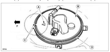
b. Align the positions of the retainer (A) and fuel pump ring (B) as shown (C), and tighten them one full rotation by hand.
