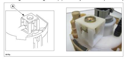
7. Perform the following procedure to install the set plate (A) to the reserve cup (B).
