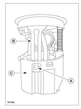
8. Route the wiring harness (A) under the nylon tube (B).
