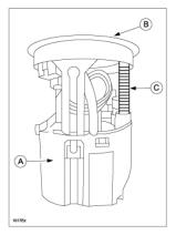
**CAUTION:** DO NOT grasp the pipe located on the upper surface of the set plate. The pipe could be damaged, causing fuel leakage.
