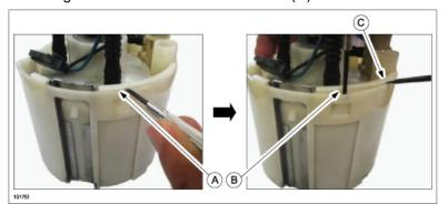
b. Pull up the fuel pump up while disengaging the snap fit tab with 2.0 mm flathead screwdriver and working the 2.3 mm flathead screwdriver (A) along the edge. Then insert the flathead screwdriver (B) and rotate to increase the gap.
