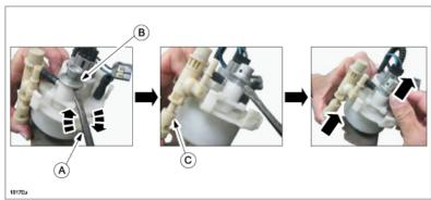
7. Remove the O-rings (A) from the transfer jet pump (B) and pressure regulator (C).
