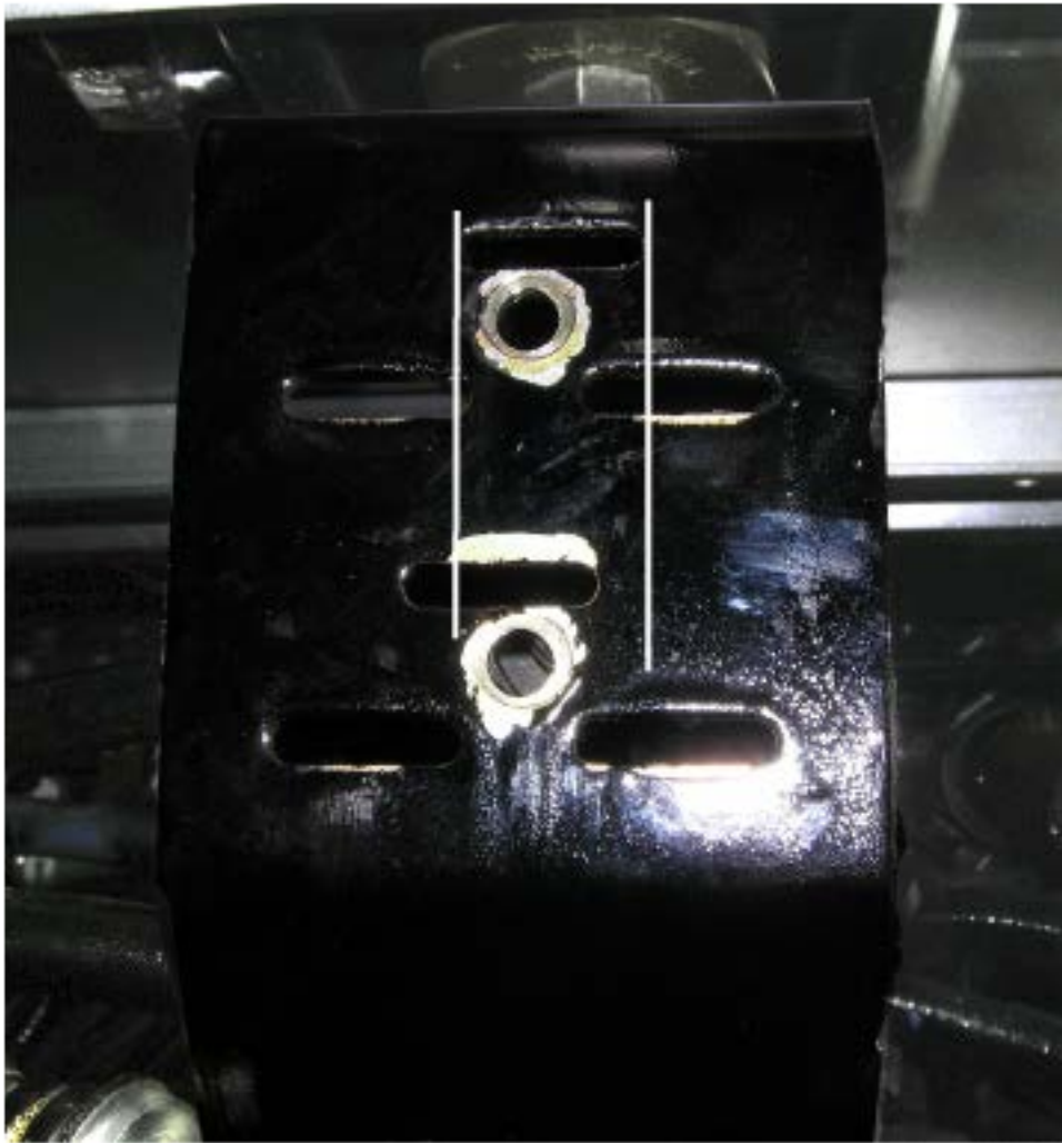
Figure 2 Fuel Tee mounting slots offset
