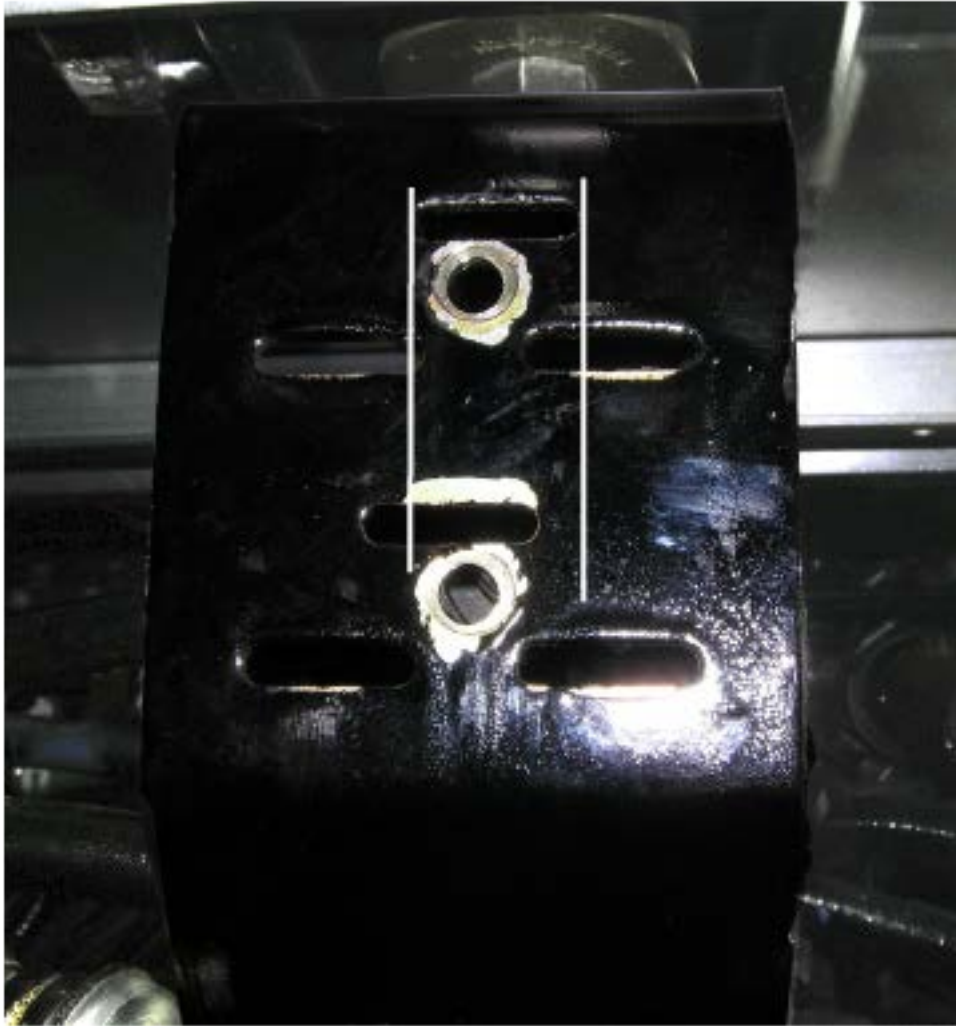
Figure 3 Fuel Tee mounting slots offset
