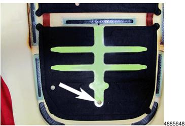
6. Center the hole in the reinforcement strip with the hole in the seat pad.
