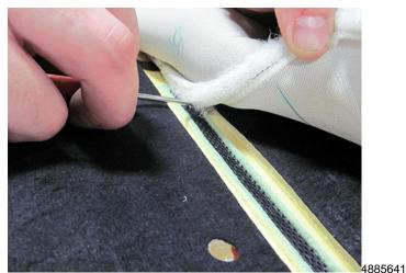
**Note:** Use a small flat blade screw driver to separate the seat cover hook and loop fastener strips from the seat foam fasteners. Do not pull the two components apart, the seat cushion may be damaged. If the cover fastener strips pull out of foam, the seat cover will not attach to seat properly, replace the cushion pad with a new cushion.
