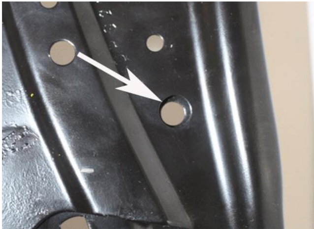
Acceptable Condition, Holes Aligned
