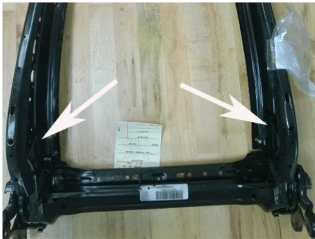
Unacceptable Condition Holes Off-Center
