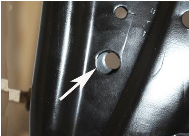
Unacceptable Condition Holes Off-Center
