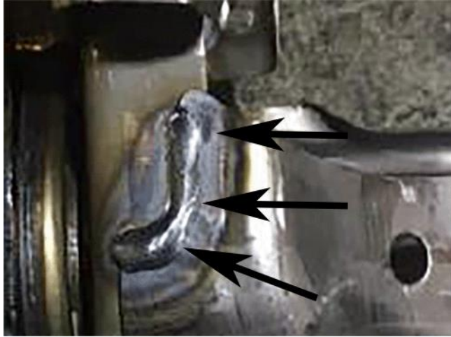
Good Weld: weld covering the edge of the bracket
