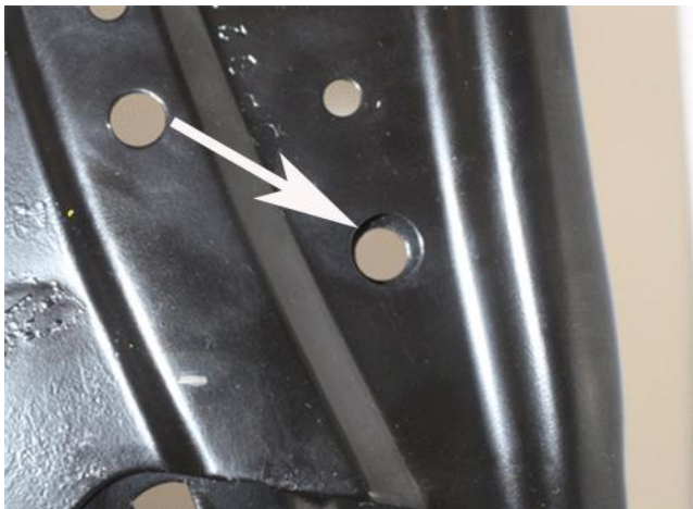
Acceptable Condition, Holes Aligned
