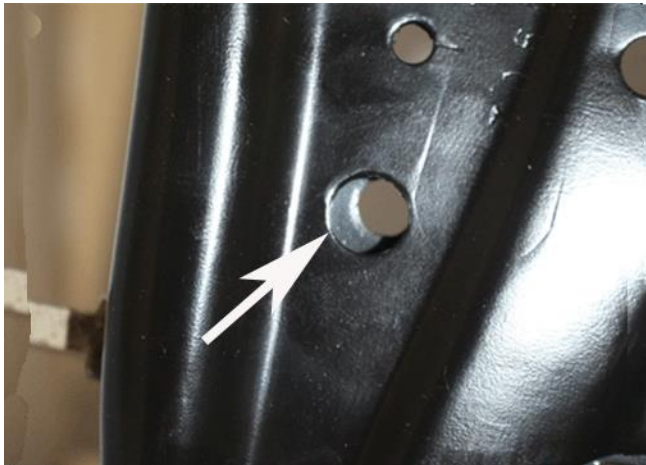
Unacceptable Condition, Holes Off-Center
