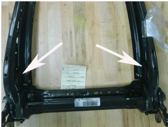
Unacceptable Condition, Holes Off-Center
