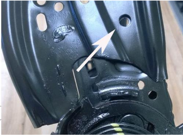
Alignment Hole Inspection Area
